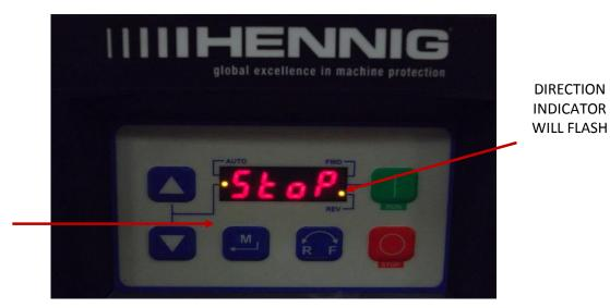
PRESS THE "ENTER" BUTTON TO CONFIRM DIRECTION
