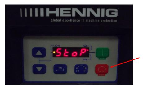
PRESS THE "SOFT STOP" BUTTON TO CLEAR FAULT
