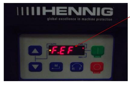
F.EF IS DISPLAYED WHEN VFD HAS COMPLETED THE POWER UP CYCLE
