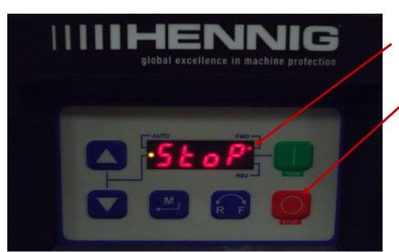
PRESS THE "STOP" BUTTON. THE DISPLAY WILL INDICATE THAT THE CONVEYOR IS STOPPED.
