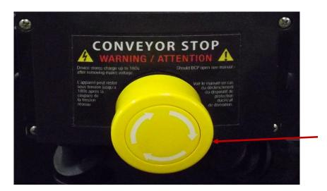
TWIST THE "CONVEYOR STOP" BUTTON TO RELEASE
