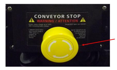
GENTLY TWIST THE "CONVEYOR STOP" BUTTON TO RELEASE.
