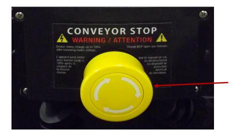
PRESS THE "CONVEYOR STOP" BUTTON FOR IMMEDIATE STOP
