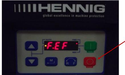
TO CLEAR THE STARTUP FAULT PRESS THE "SOFT STOP" OR CLEAR FAULT BUTTON
